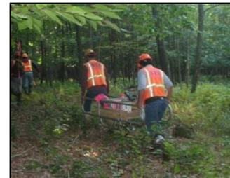
The Sled arrangement with two people carrying the unit provides a stable platform so that the inertial navigation sensor gives much better real-time and post processed results than the Backpack mode. Trip-and-fall incidents are virtually eliminated making this the safest operation mode preferred by some of the most demanding clients.
